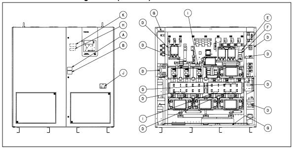
Figure 2 - UPS exterior/interior showing warning labels.
